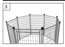
3 Repeat these steps until you have an octagonal shape. Make sure the Kennel Gate Panel and Latching Window Panel are placed where both panels can be opened from the outside.
