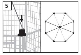
5 Insert the end of a Roof Support Arm into the second hole of the Nylon Panel Connector.
