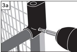
**3a**To turn your **Pet Gazebo** into a semi-permanent structure (optional), use a power drill and screw the **Self Tapping Screws** into the predrilled holes provided on the connectors.
