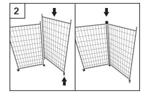
2 Place a Nylon Pannel Connector on to one side of another Kennel Wall Panel and insert the second Kennel Wall Panel into a Nylon Panel Connector of the first Kennel Wall Panel.
