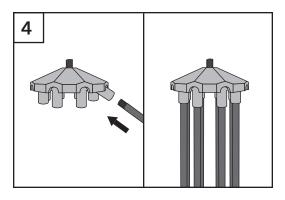
4 Insert the tip of the Roof Support Arm into the sleeve of the Roof Hub and screw into place by turning the Support Arm to the right (clockwise). Screw the arm in completely and make sure the angled end of the Roof Arm is pointing in towards the Roof Hub.
